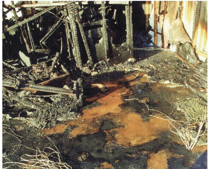
*Figure 1: Irregular burn patterns on the floor created in a test fire where no accelerants were used. (Photo: Scientific Protocols for Fire Investigation, John Lentini, pg 487)*
