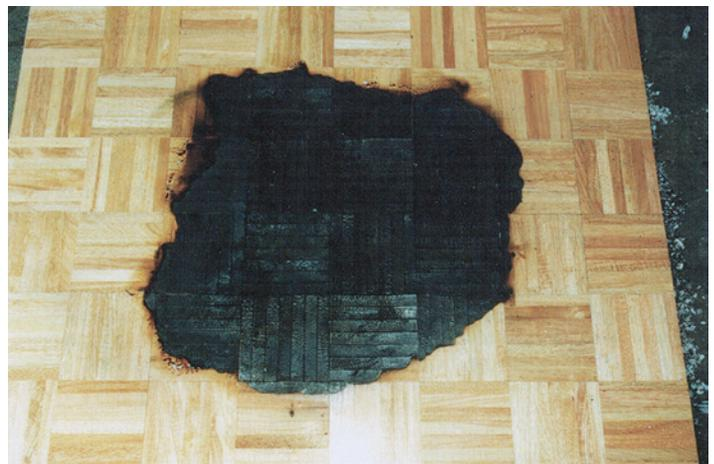
*Figure 2: Puddle-shaped burn pattern created by burning a cardboard box on an oak parquet floor (Photo: Scientific Protocols for Fire Investigation, John Lentini, pg 484)*
